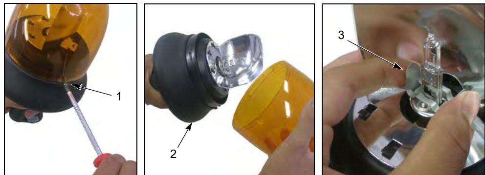
Fig. 8-5 Replacing the bulb
