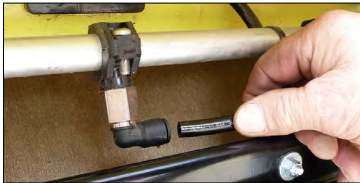
Fig. 11-1 Draining sprinkling water
