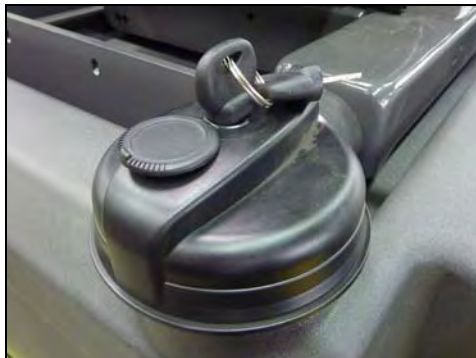
Fig. 8-9 Water tank cover
