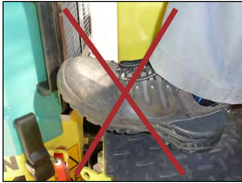
Fig. 7-2 Danger to foot of crushing
