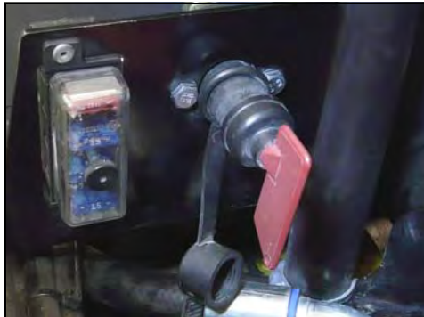
Fig. 8-11 Switching off the power
