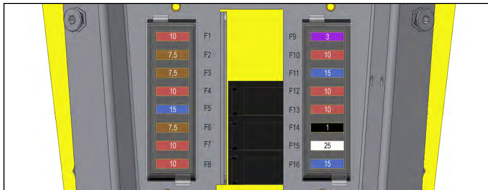
Fig. 10-5 Position of fuses in the steering column
