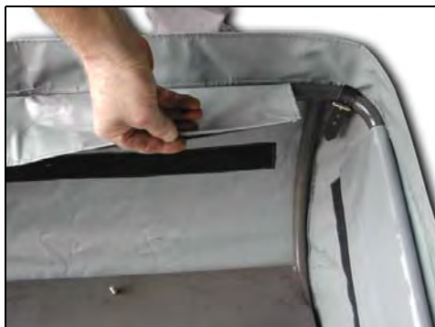
Fig. 8-6 Removing the tarpaulin
