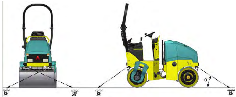
Fig. 12-4 Lashing the roller / side view
