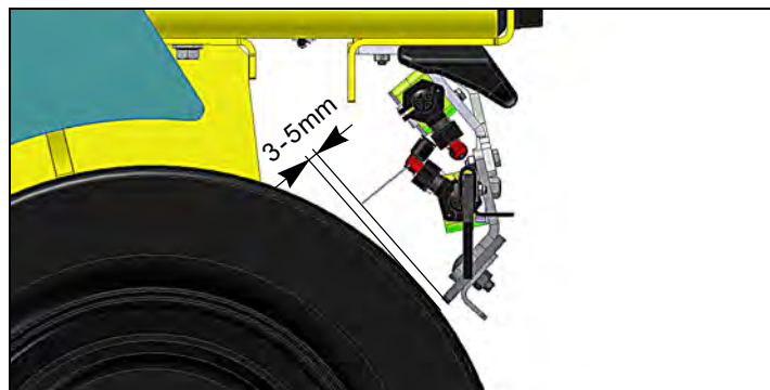
Fig. 9-24 Clearance of scraper to pneumatic wheels
